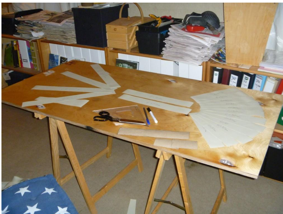
20150101 The pocket gap cover strips of Ingeborg's sail. All of them are 60mm wide. This temporary table was very helpful for such small jobs...
