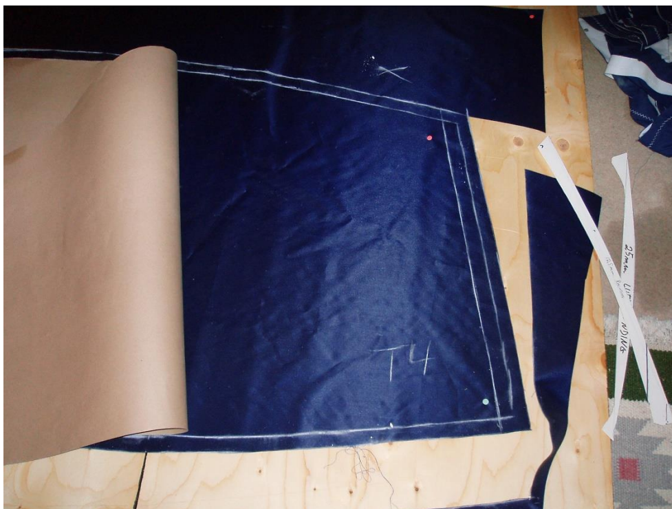
20090218 Detail from making Broremann's sail. A 20mm "frame" around the "net size" pattern has been added to the cloth. Note the extra helping line at the luff. Handy when putting on the hem...
