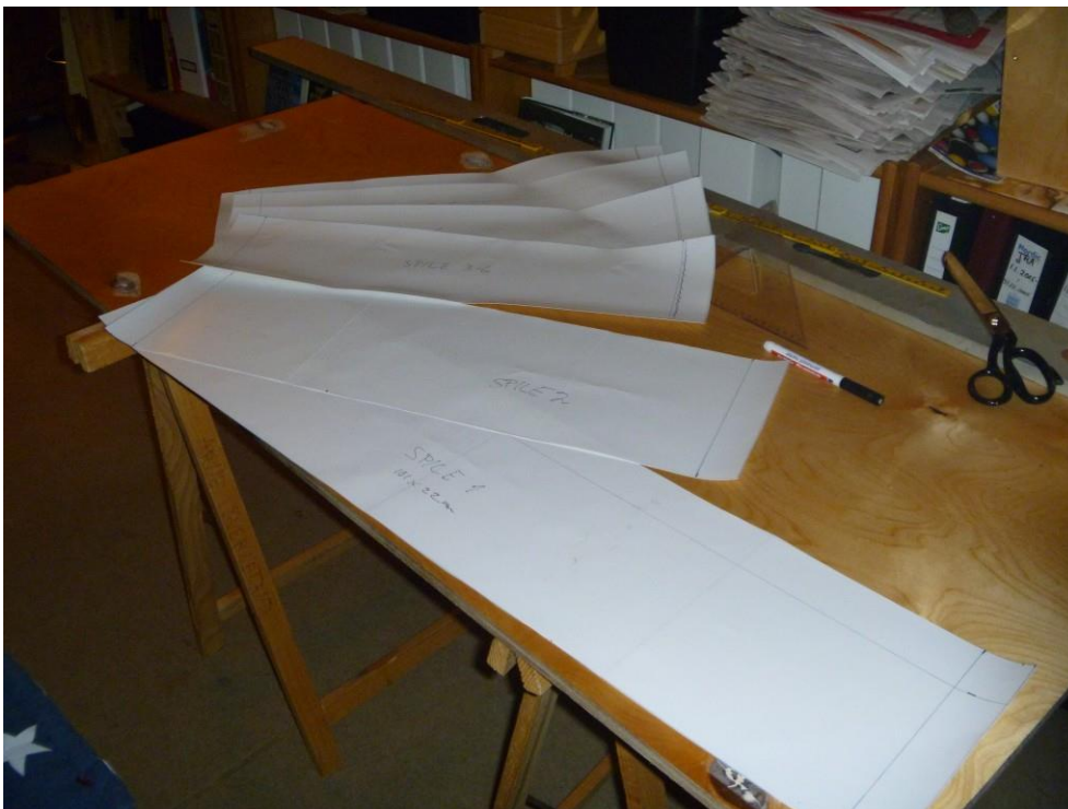
20150102 The forward batten pockets for Ingeborg's sail, made of thick PVC material. They are made ready for 20mm hems at the end.
