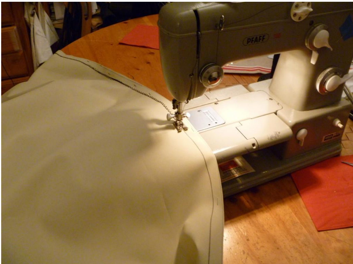
20141230 joining two batten panels with the Batten Panel Joining Seam . Easy...
