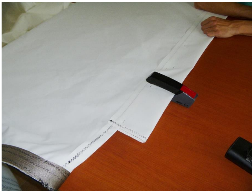
20120610 Stapling on the aft batten pocket on ED after the cover strip has been sewn on.
