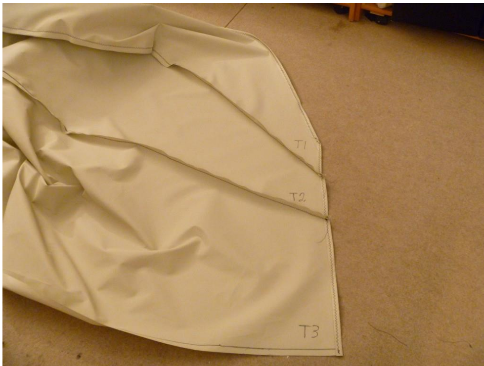
20150106, Ingeborg's sail: The assembled but still naked top section marks the end of STEP 3....
