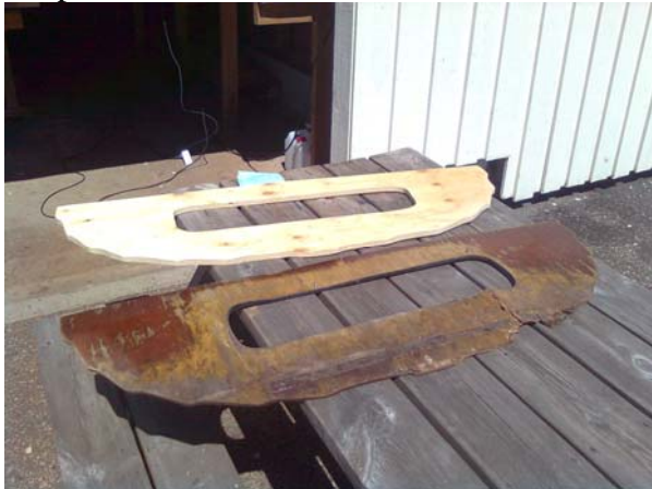
.. the old and the new bulkhead..
