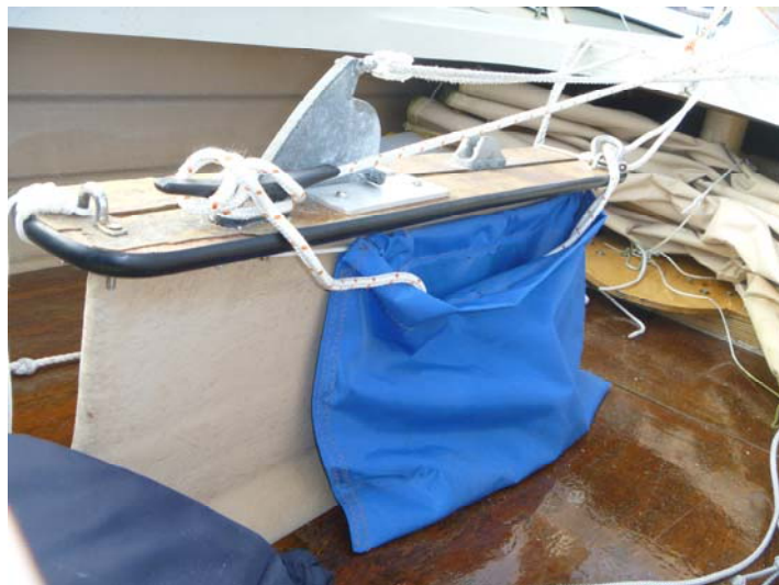
The halyard and running parrels share a bag. Practical as their tails are not long at the same time.
