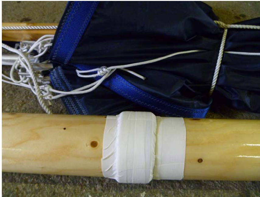
..the mast, coated with 5 coats of 2-pot varnish from Epifanes. The waistbelt at deck level taped in place...
