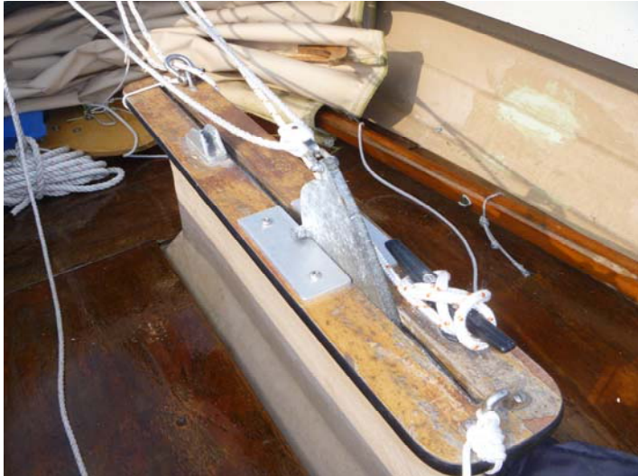
Over the years the stop-bolt in the centre board had chewed its way through the plywood so two pads of aluminium was fitted. The halyard is cleated to that black cleat on the c.b. trunk. Easy to reach...
