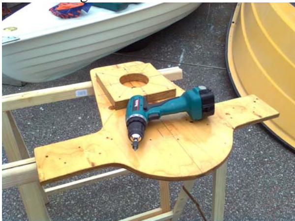
.. mast-step being readied for test fitting..
