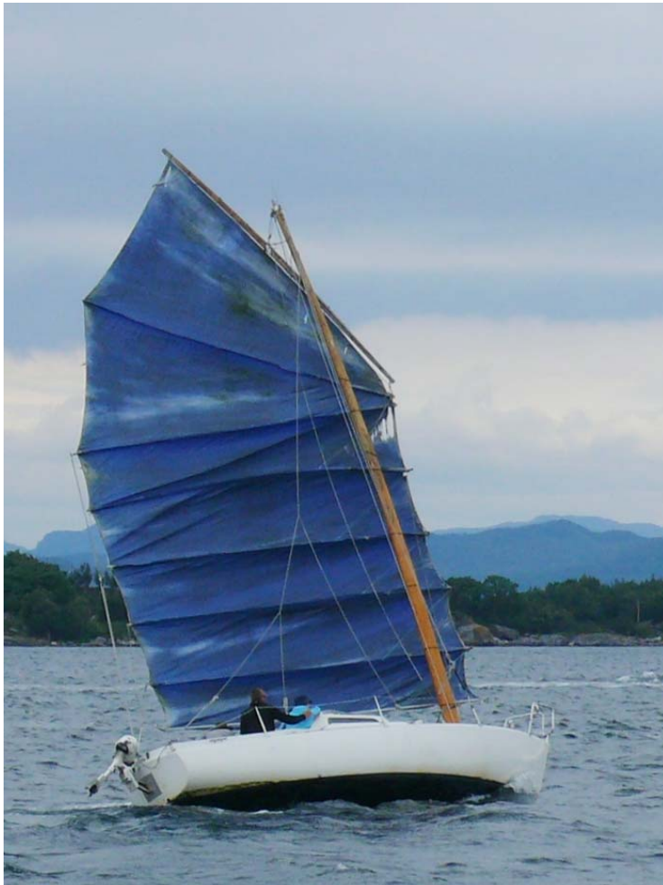
Photo 4: August 2010. Batten no. 3 clearly being bent upwards by the HK parrel in a good breeze. (Photo: Andrew Bailey)
