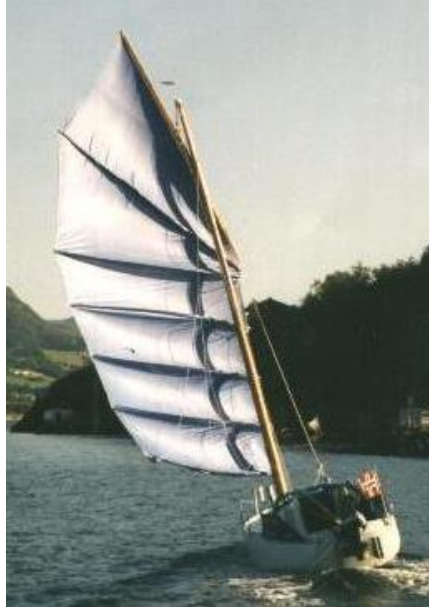
Photo 3, summer 1994: Brand new sail - and already a moderate bend visible in batten no. 3 Photo: Reidar B Kalvig
