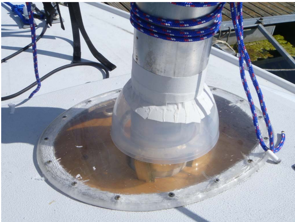
25.7 The partners may look odd, but it seems to work, and it keeps the rain out...
