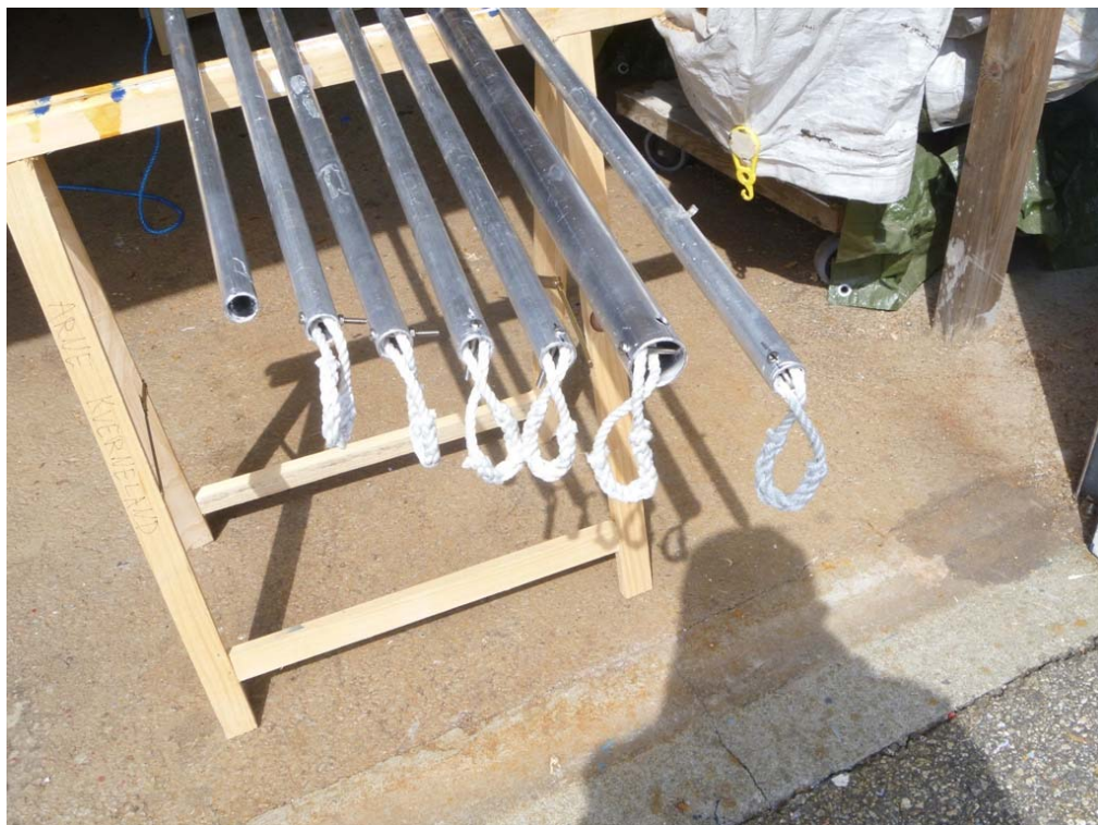
13. Mai Preparing the battens. Most were 22 x 2mm but batten 3 is 35 x 2mm (all 6061-T6 alloy)
