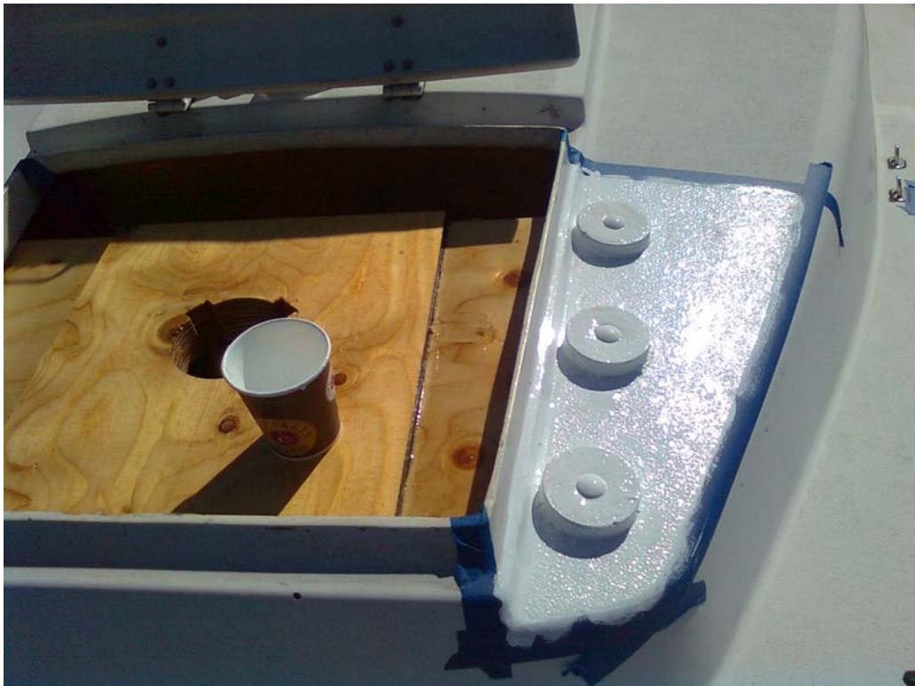
20.July The partners was a also a plywood job, glued and bolted on. The hatch takes no loads.
