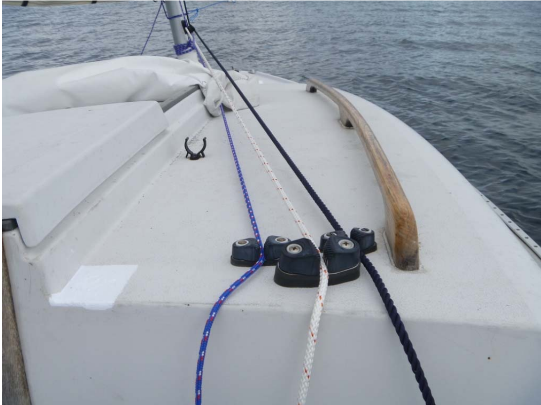
..simple setup, from left to right, Yard h. parrel, halyard, throat hauling parrel...
