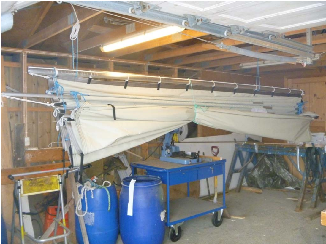
16. July. Mating the sail with yard and battens indoors proved to save a lot of time...
