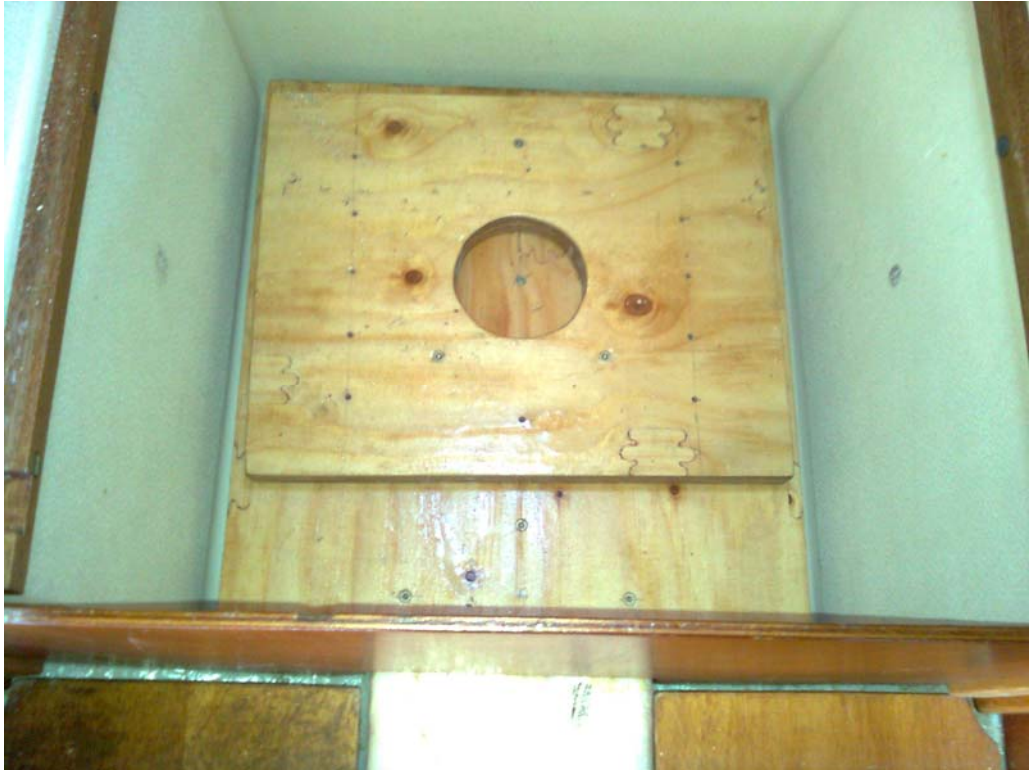
12. 7 The mast step consists of a thick plywood base, onto which the maststep is just screwed on.
