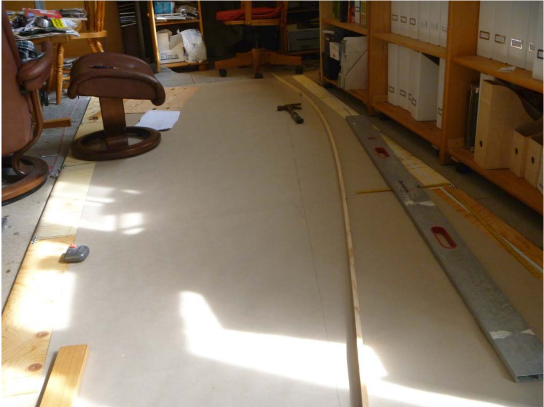
17. April. Making a paper template for the 4 lower panels. A wooden spline is used for getting the right “barrel” round.
