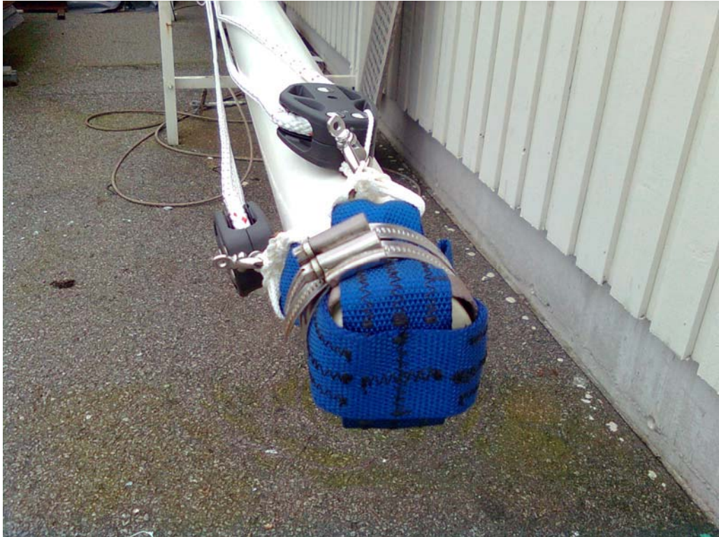
13. July The mast dressed up with halyard etc. The mast cap is stitched together from thick webbing and held in position with 2 hoseclamps.
