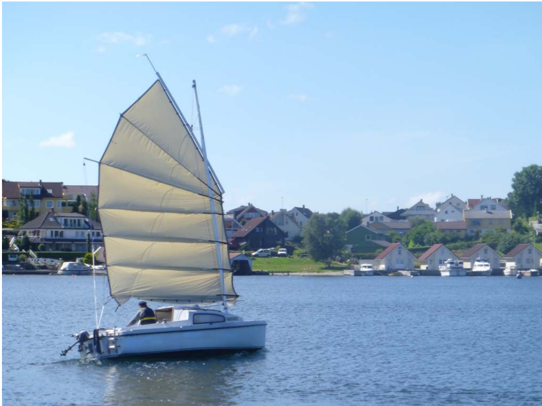
.. FS is super-easy to manoeuvre. Note the yard extension with a piece of sail cloth added to tell the wind. Up there the wind is not disturbed by the sail.
