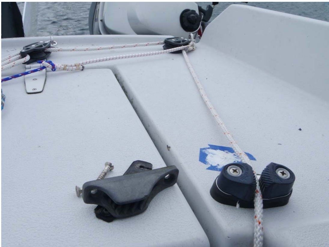
.. and here the sheet. The cleats used have mainly been picked from the cockpit coamings...
