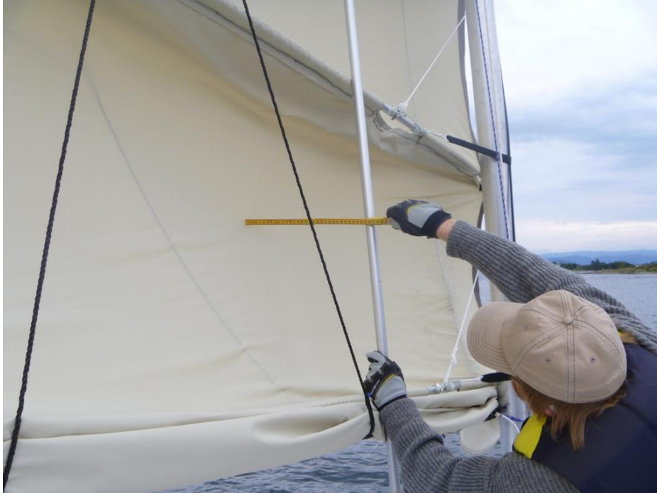
.. 6.9: Measuring the real camber...
