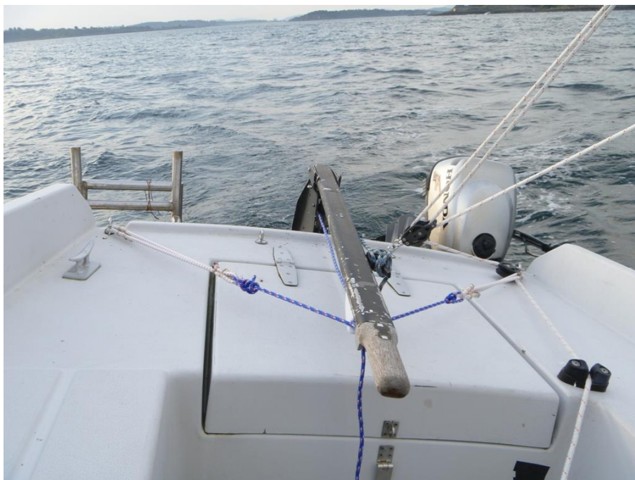
.. 23.8: The tiller brake at work along with the Honda at rest. The sheet is easy to release...
