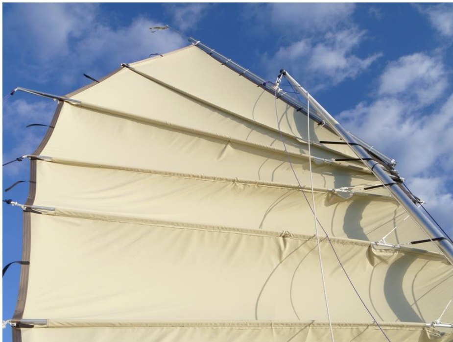
.. 27.8: The shadows, cast by the mast, illustrate the vertical camber from batten to batten...
