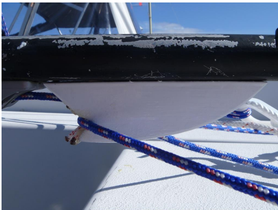
.. 3.9: Tiller brake detail...
