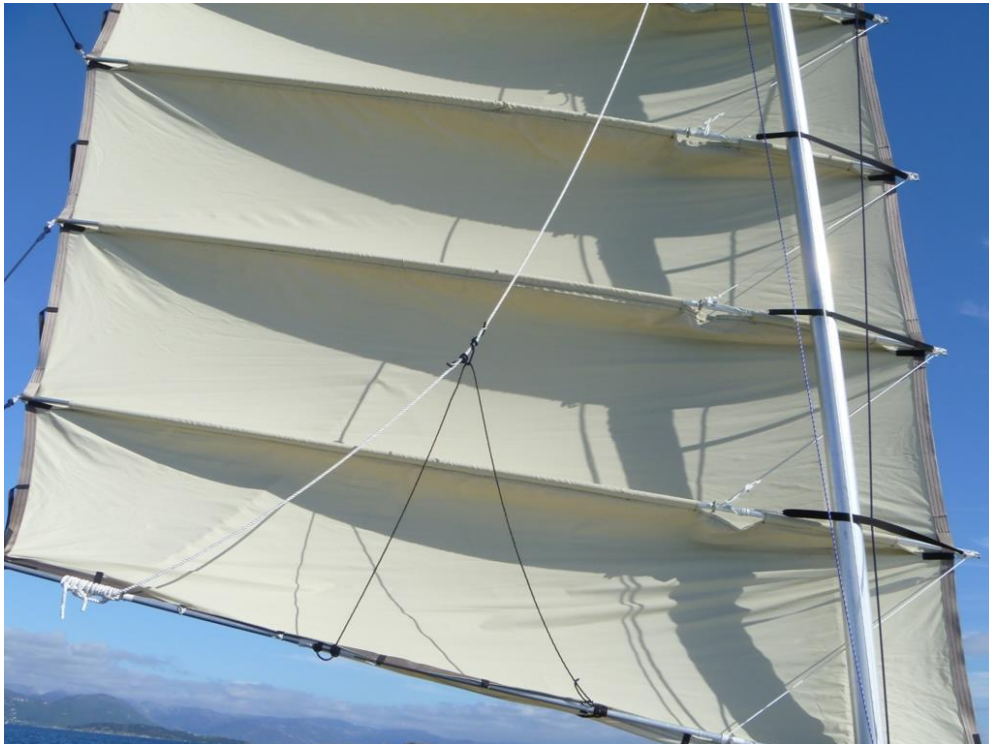
.. with the higher sun and a full sail, stretched by the elastic tack line, the sail looks as it should...
