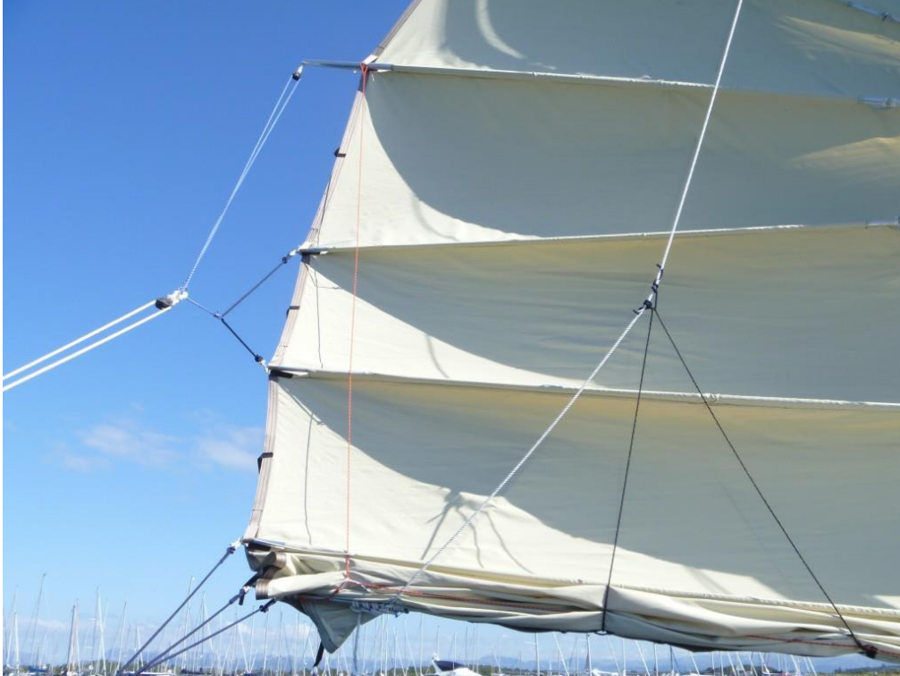
The sail has just been set with only 5 panels up. The thin, red FUP-line can just be spotted.
