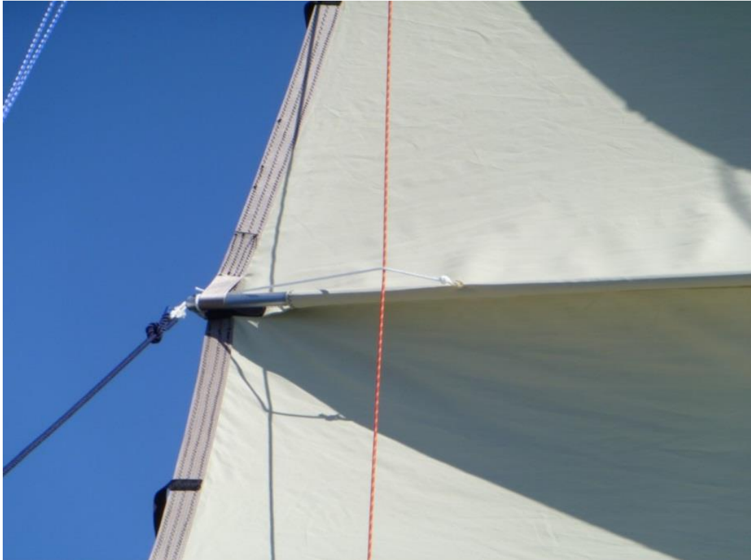
Here an aux. batten parrel can be seen, keeping the FUP line under some control, when slack...
