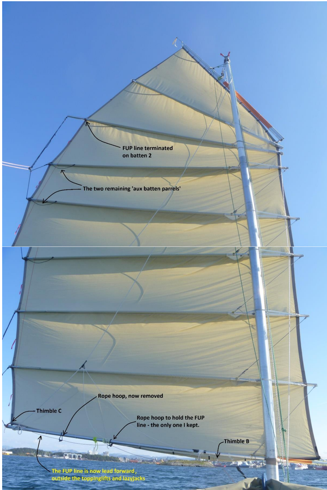
20180904 Details around my FUP MkIb setup in Ingeborg (.. note - the sail has only 7 panels...)
