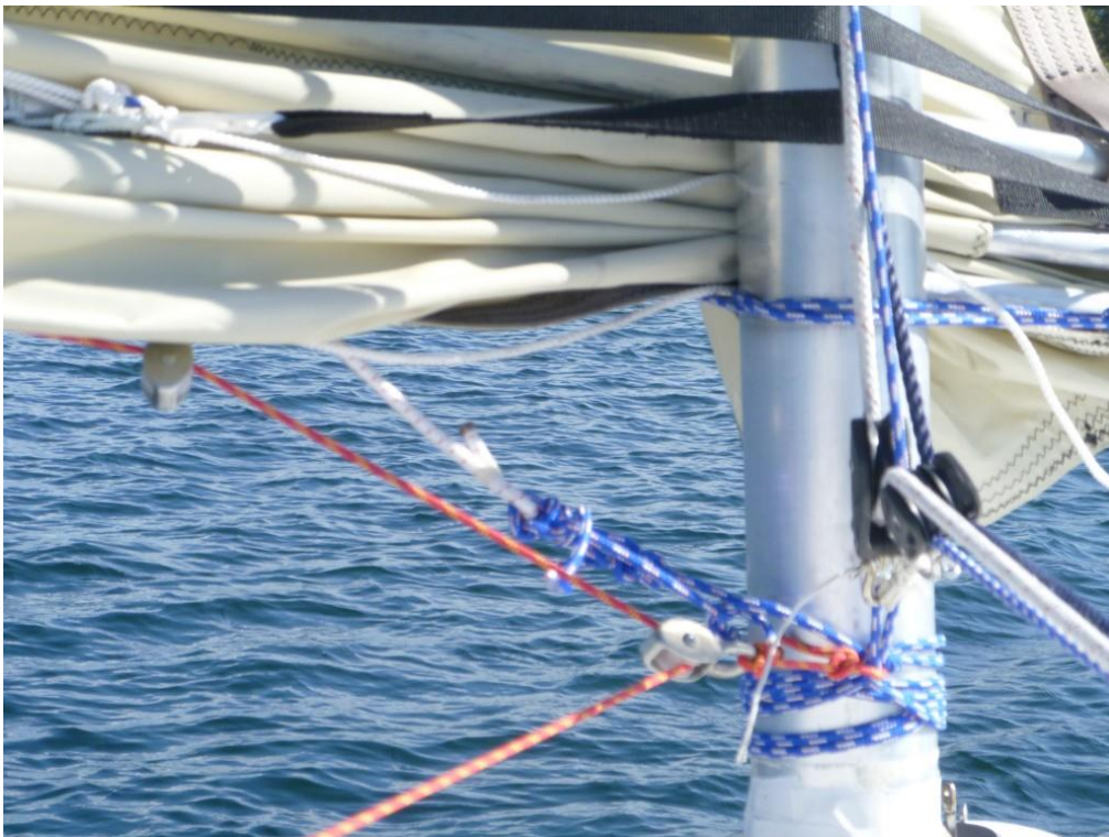
The red 4mm FUP line passes through block A and B, and thus provides some kicking strap effect
