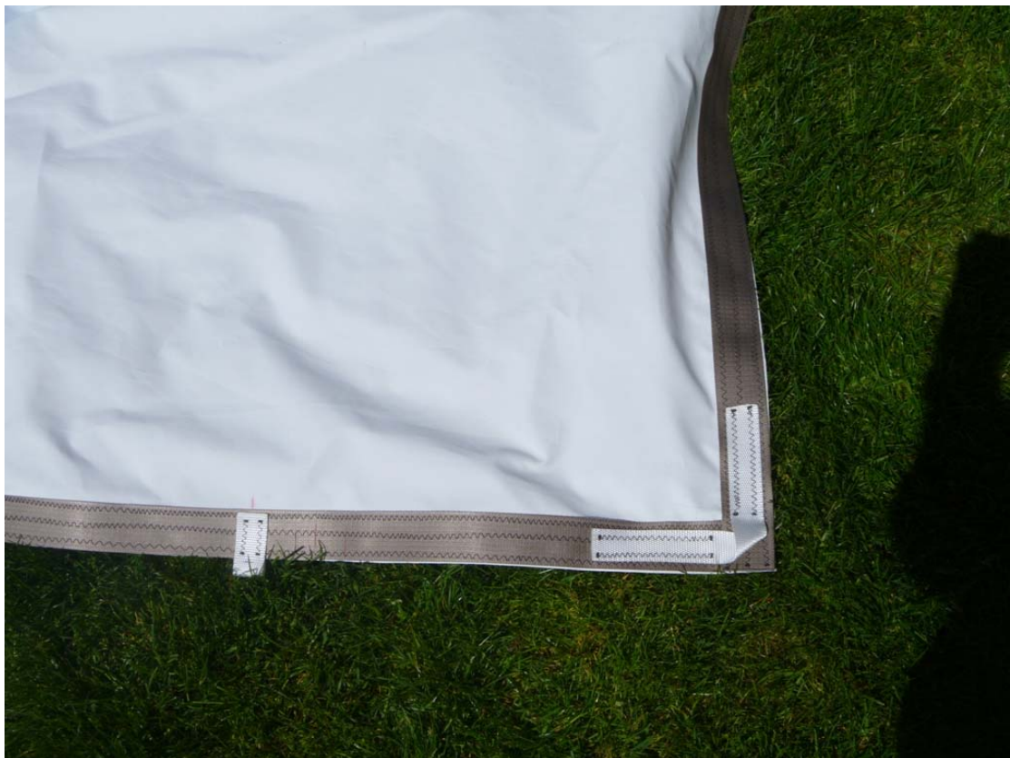
.. the tack. Small loads here so only light webbing is used for the loop...
