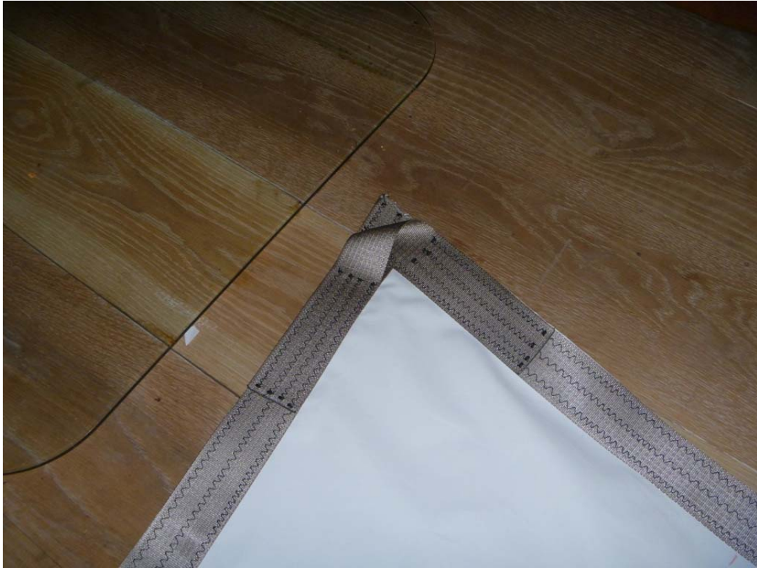
.. this quadruple-stitched loop was fitted to the peak...
