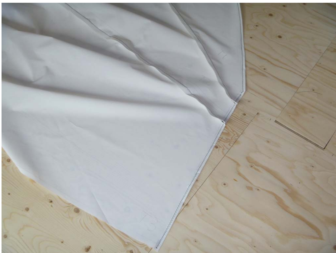
.. here panels 1 – 3 have been assembled. This is step one in the Amateur Method B in the “... Making the Sail ” chapter. Before that assembly job, the outer edges of each panel had been given a simple 20mm hem. Later the webbing boltrope was fitted...
