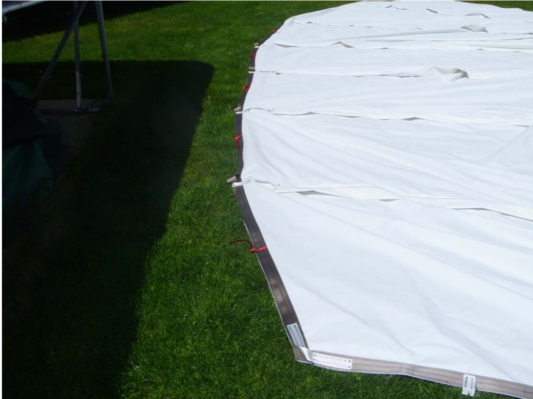
.. the clew and lower leech. Here too I used a light webbing for the hoop...
