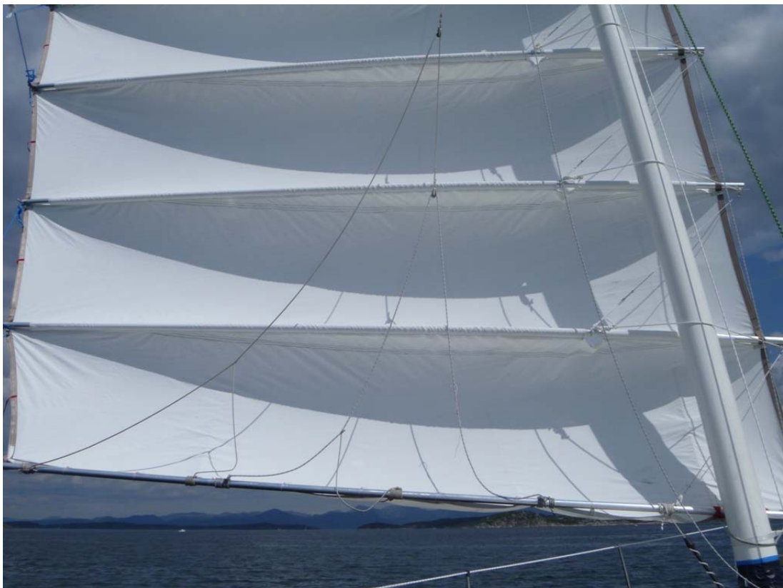
... thanks to the sunshine, the 9% camber can be spotted without much difficulty...
