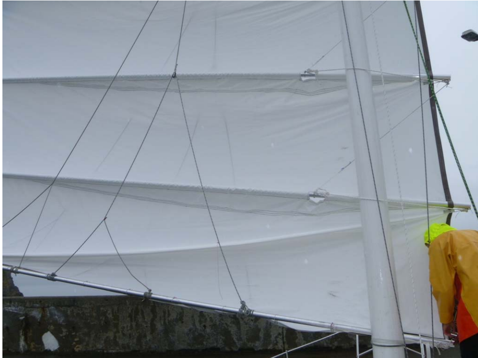
..all HK parrels fitted except to the lowest panel..
