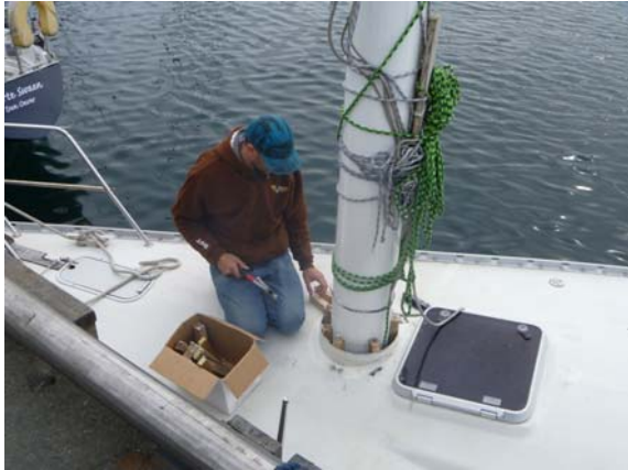
15:29, time for installing the wedges...
