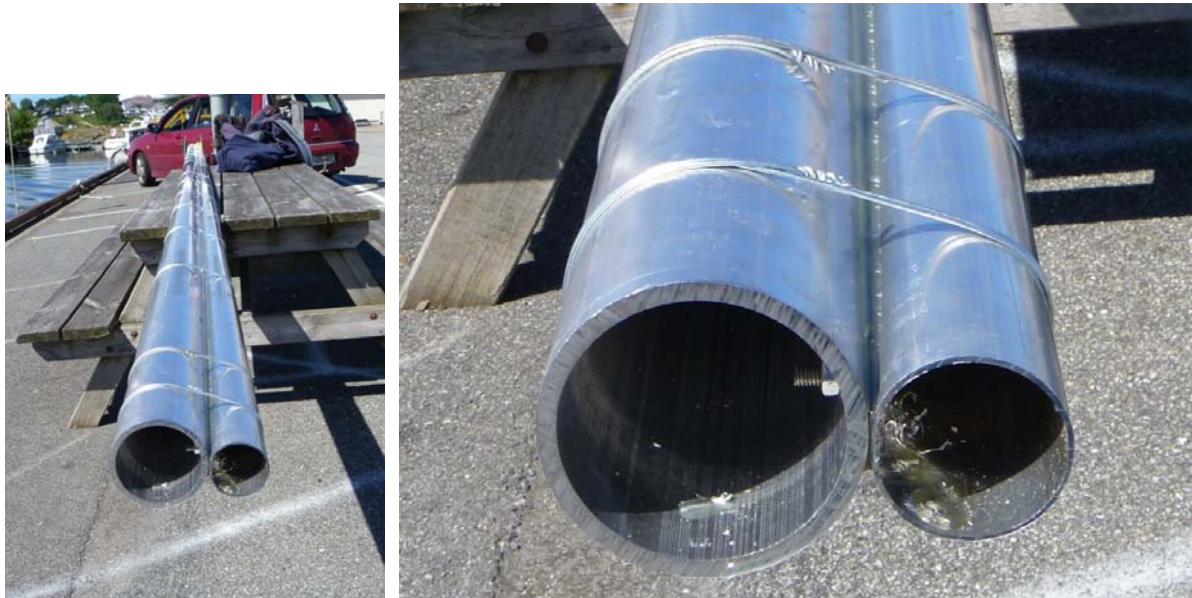
The yard; one 80mm plus one 50mm tube tied, glued and bolted together..
