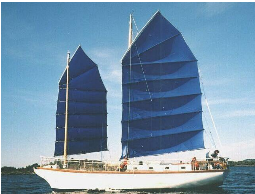
.. Samson in September 2000, 70 + 37m 2 sails. The sailplan was drawn in 1993(!) so this was before the Johanna sailplan with 70° yard was thought of. However, since the sail was made in 2000, the cambered panels were incorporated - 10% camber in the foresail and 8% in the main...
