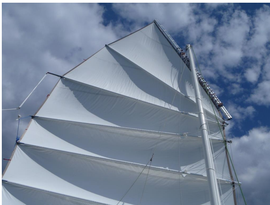
The 48\text{m}^2 sail of Edmond Dantes , made of white 6.5oz Odyssey III
