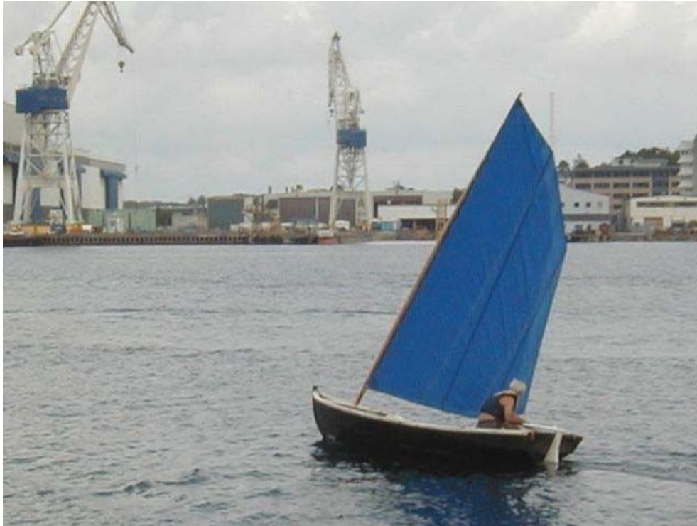
.. Curtiss with his Lj-rigged rowboat (LOA=4.9m, SA =7.4sqm, mast 5.5m/7.0cm)..
