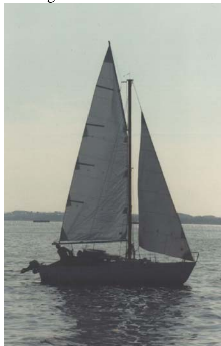
The 23' Albin Viggen, Malena with a gaff mainsail fitted in 1985. Note the position of the 3 rd reef...
