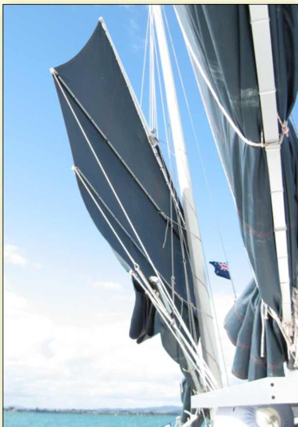
Fan camber pulling well, on starboard & port tacks
