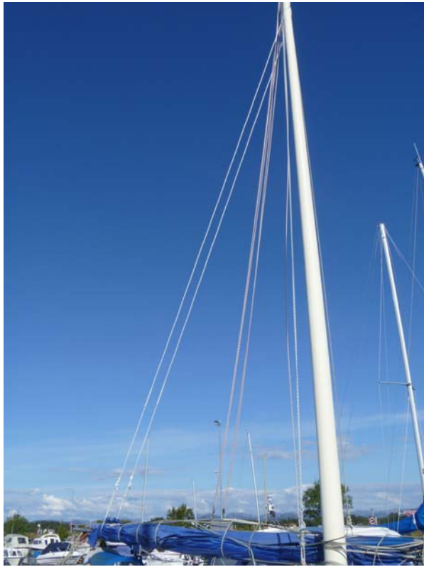
.. The main part of the LJ in place. The sail ties keep the bundle tidy until the sail catchers are fitted....
