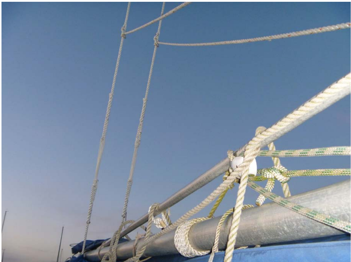
.. the “cables” for the sail catchers fitted. Note the approx 20cm spans on the topping lifts, held together with lacing between spliced eyes. These let me do fine adjustments (in harbour). After a month’s use I shortened these to compensate for stretch...
