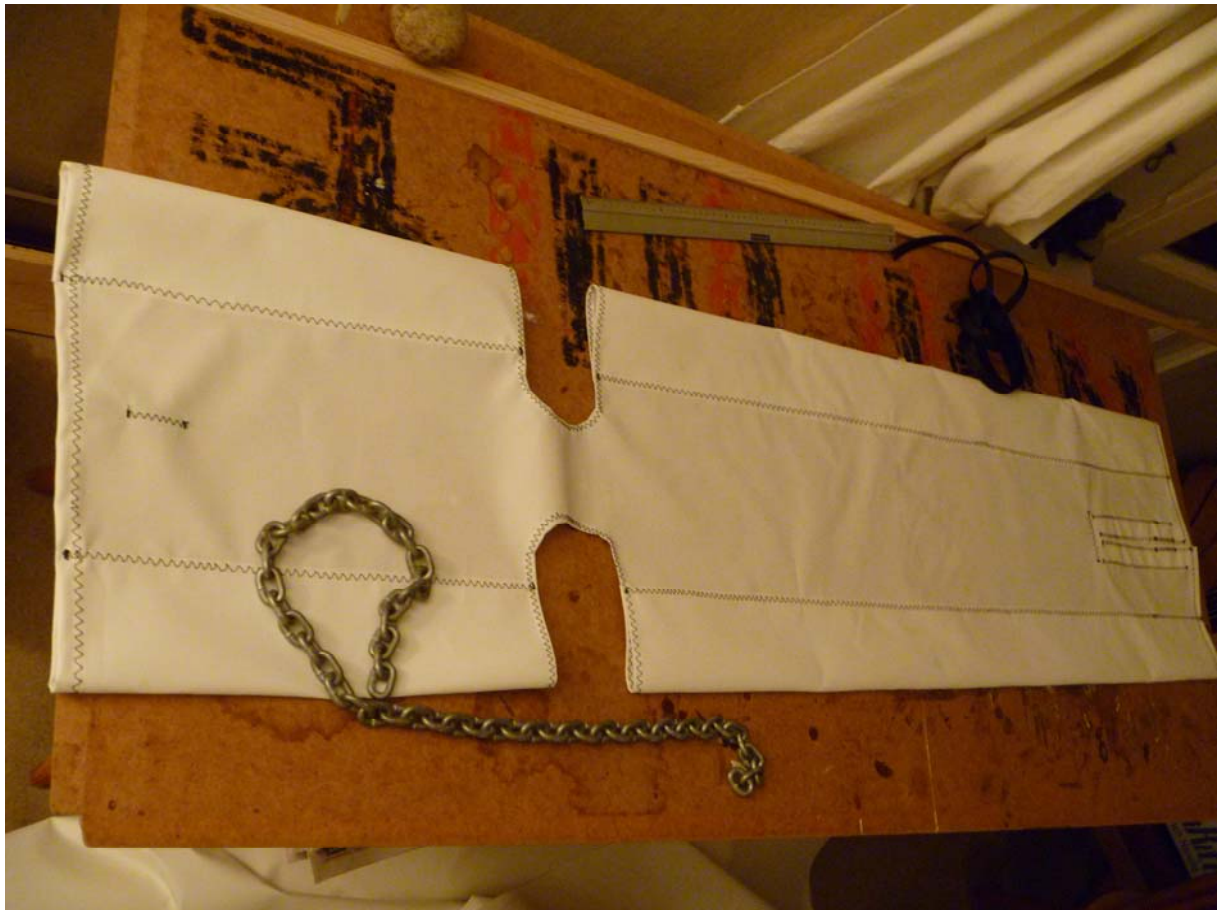
..the fore part of Broremann's sail cover, prior to inserting the chain in the wide side hems. Note the big cut-outs for the mast and mast lift and the central slot for the halyard far to the right...
