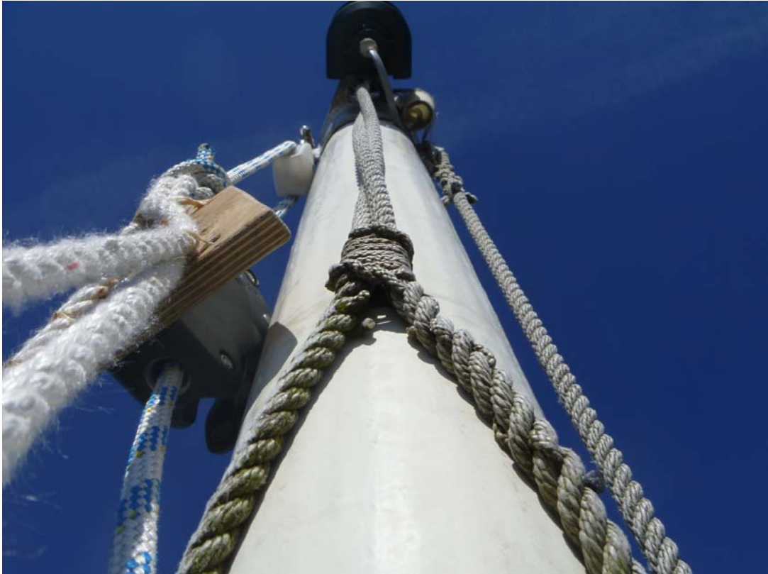
..looking at the masthead; the old LJ still in place. The new LJ is rigged in the same way...
