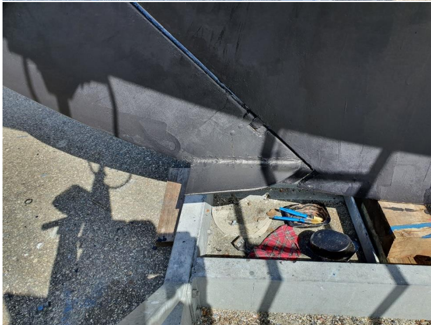
20200723: The endplates, epoxied on, painted and ready for launching.
