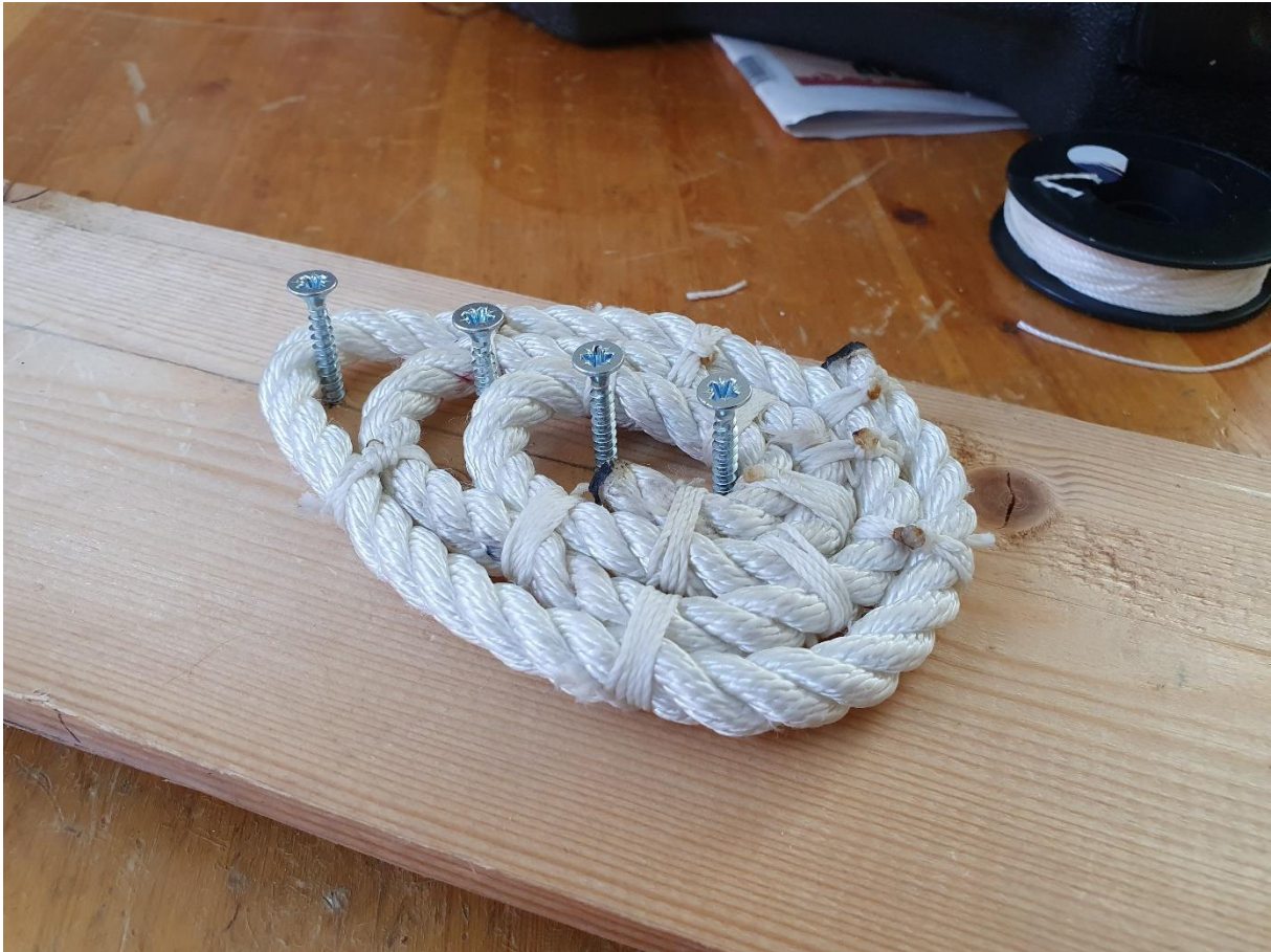
..stitching and seizing together a 3-hole soft euphroe...
