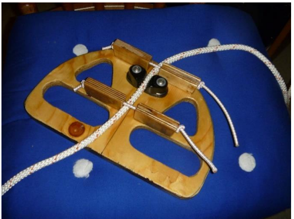
..the Halyard Hauler Mk.3, with a stock camcleat...
