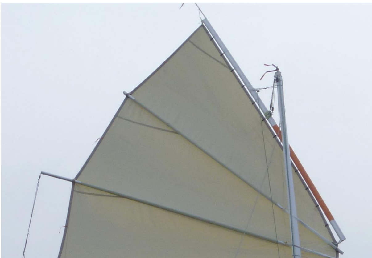
20190611 The 5-part halyard on Ingeborg. The forward slingpoint has slipped aft a bit.
