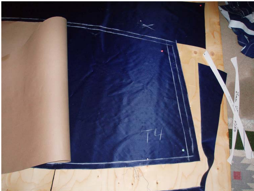
.. panel 4 ready with tack corner marked on. No luff rounding here...
