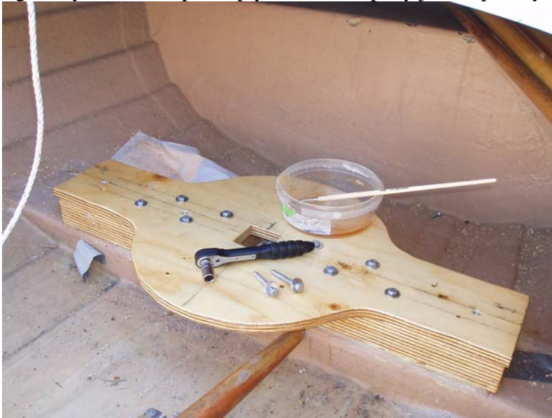
.. maststep, the top is just screwed on for easy removal...
