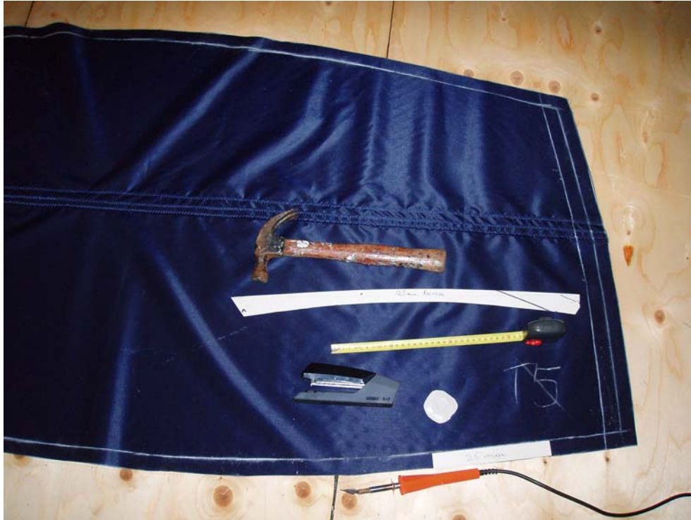
..panel 5 cut out and marked up for sewing. Note the handy 25mm spacer, next to the hot-knife...
